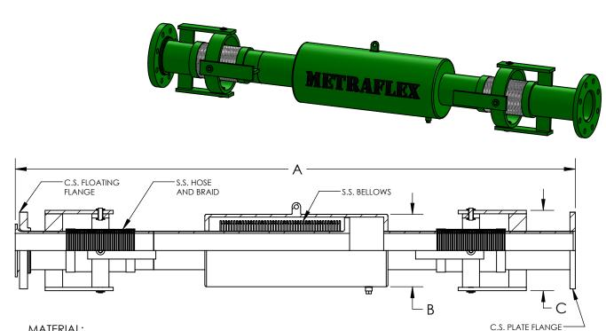
MATERIAL: BELLOWS - MULTI-PLY STAINLESS STEEL HOSE AND BRAID - STAINLESS STEEL OTHER PARTS - CARBON STEEL
